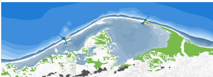
Figure 6. Phase 1 of the Bardawil Development Project consisting of the dredging of Boughaz 1 and Boughaz 2.
